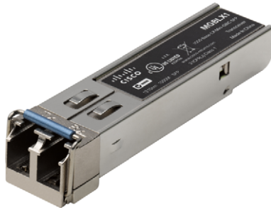
FIGURE 7.2 SFP+ for fiberoptic Ethernet
