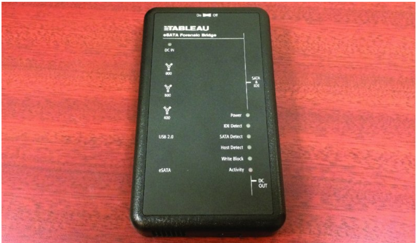
Figure 7.8 A Tableau SATA- and IDE-capable hardware write blocker
