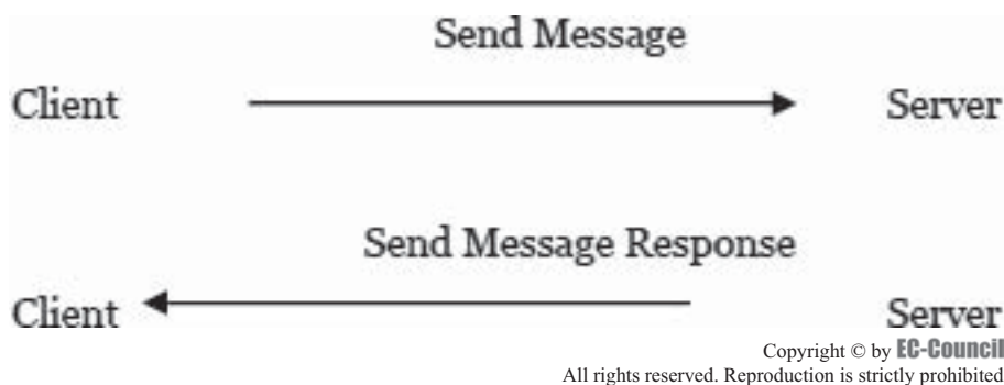
Figure 3-12 The client initially requests a connection by sending the URLConnection message to the server. The server replies to the request and closes the connection. www.hellodigi.ir
