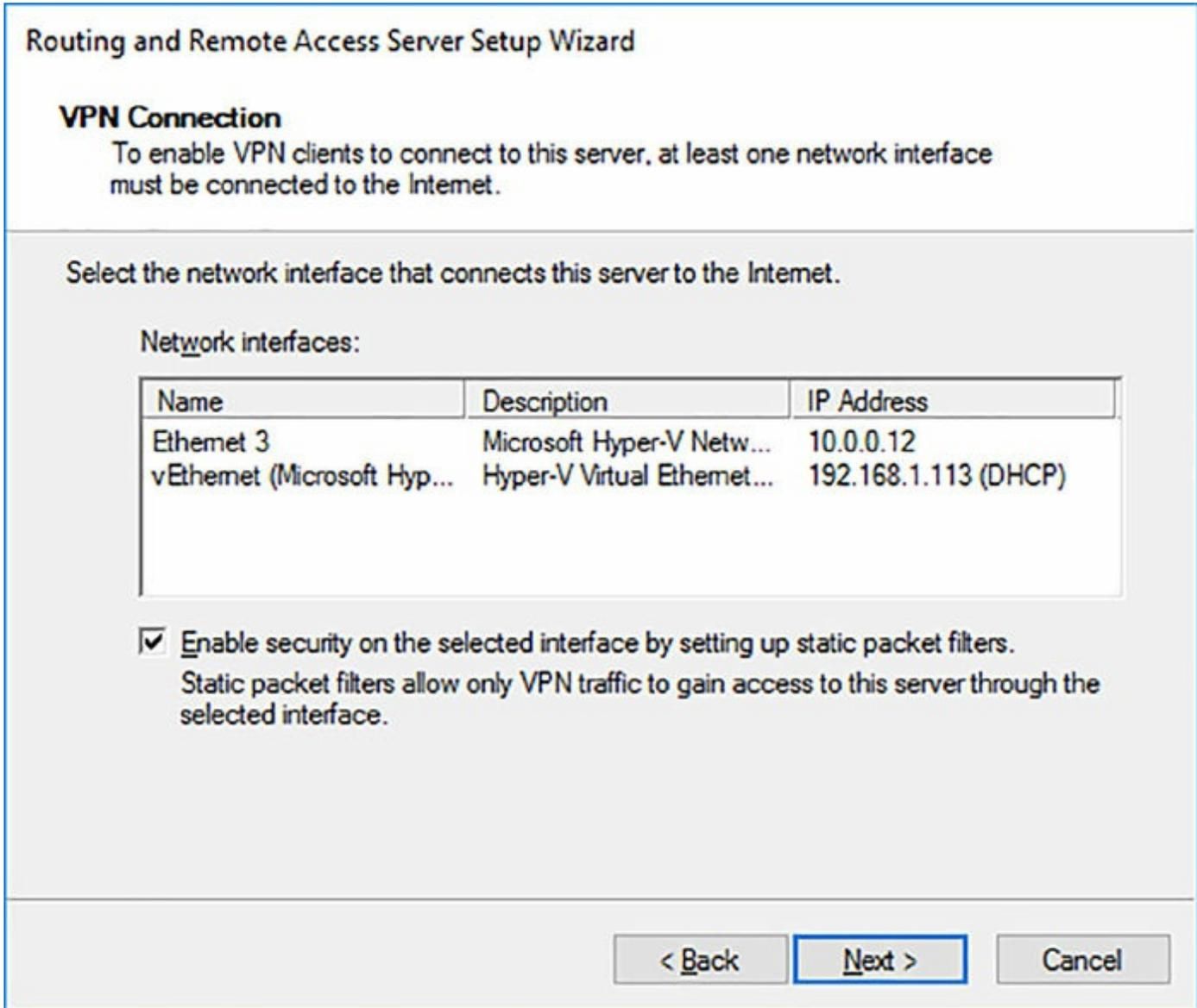
**FIGURE 8-4** RAS Setup Wizard VPN Connection
