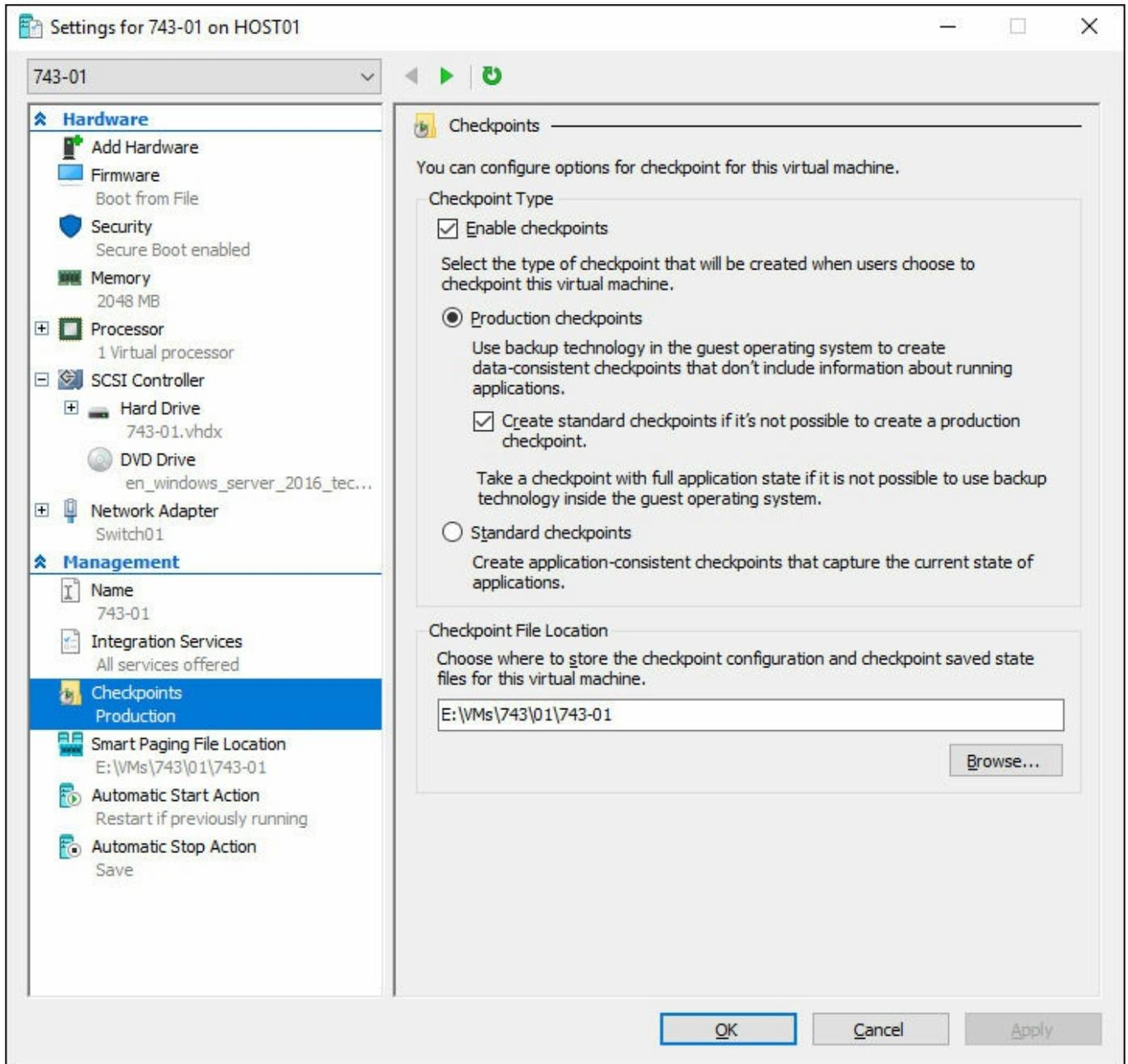
**FIGURE 3-20** Virtual Machine Checkpoint Settings
