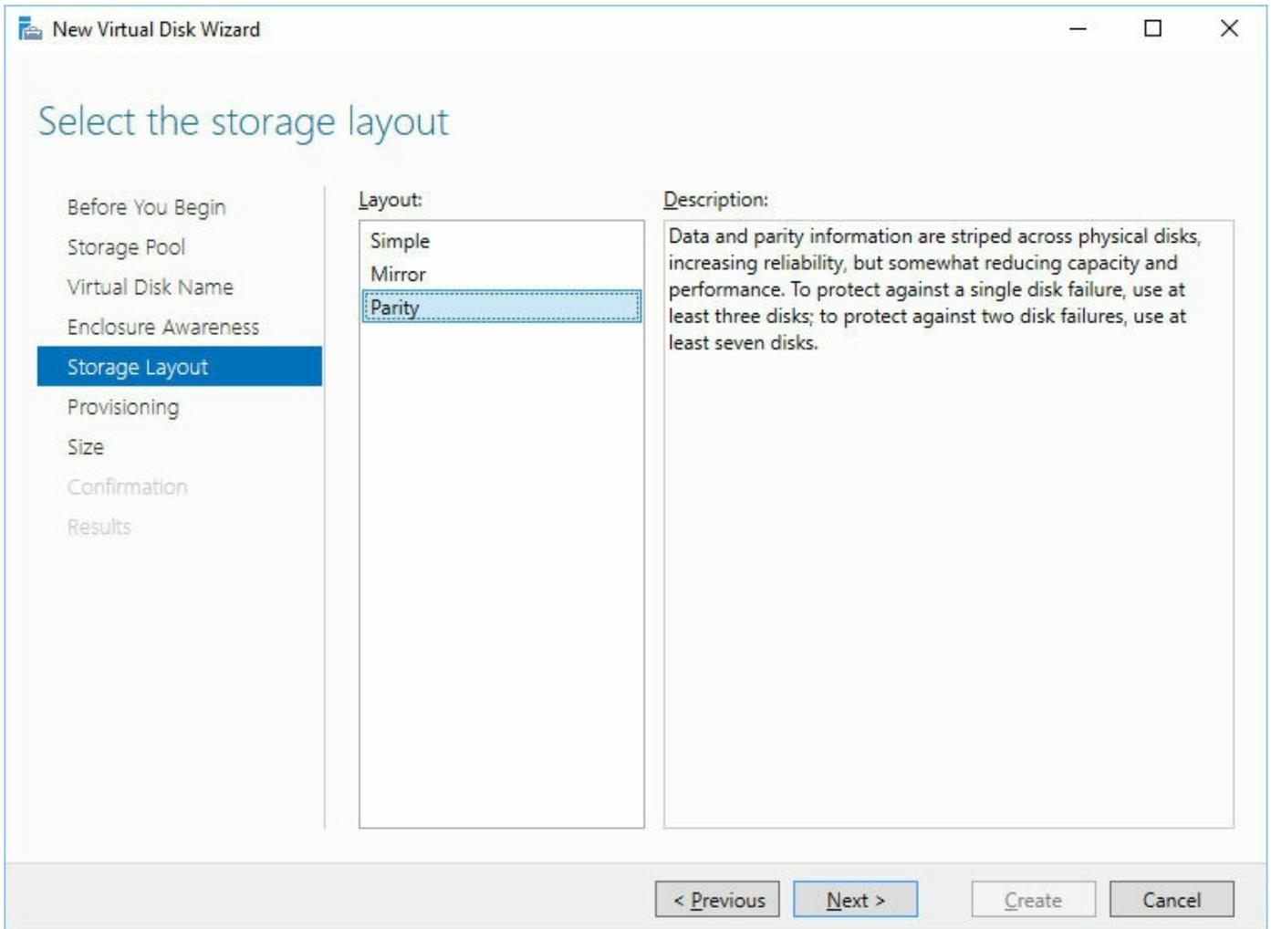
**FIGURE 2-5** New Virtual Disk Wizard, Storage Layout
