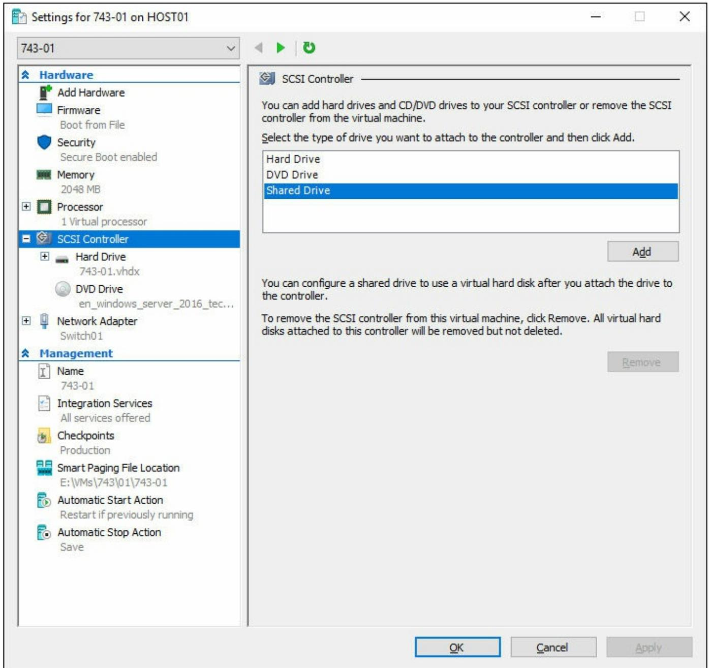
**FIGURE 3-15** SCSI Controller Settings for a VM
