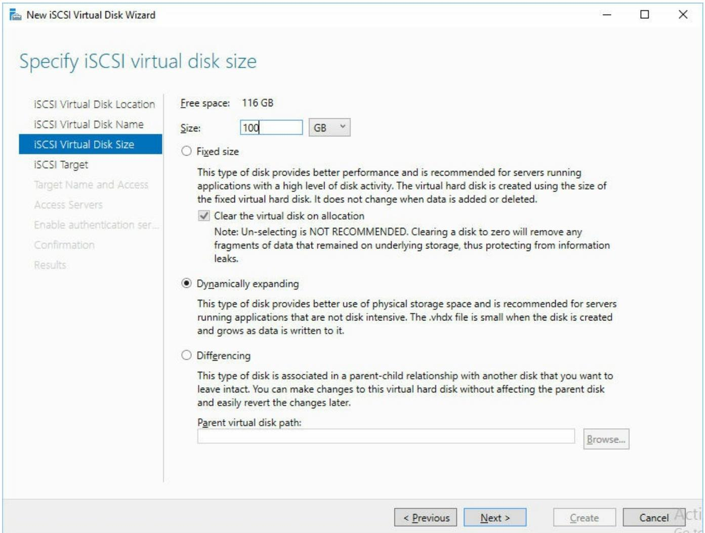
**FIGURE 2-8** iSCSI virtual disk size
