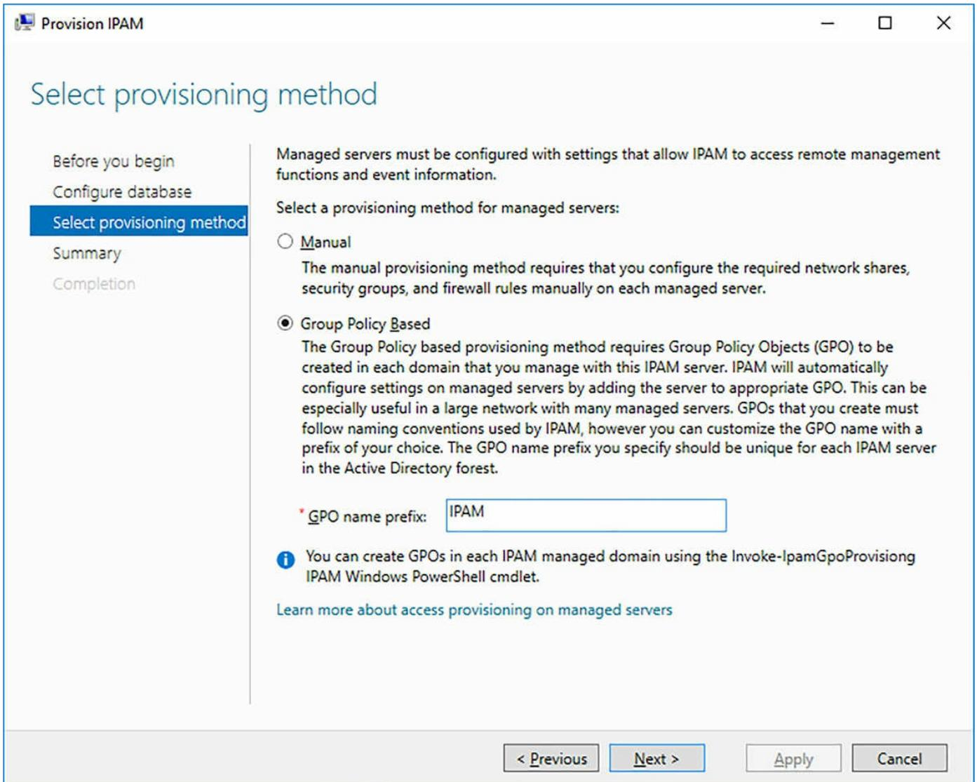
**FIGURE 7-2** Selecting the IPAM provisioning method
