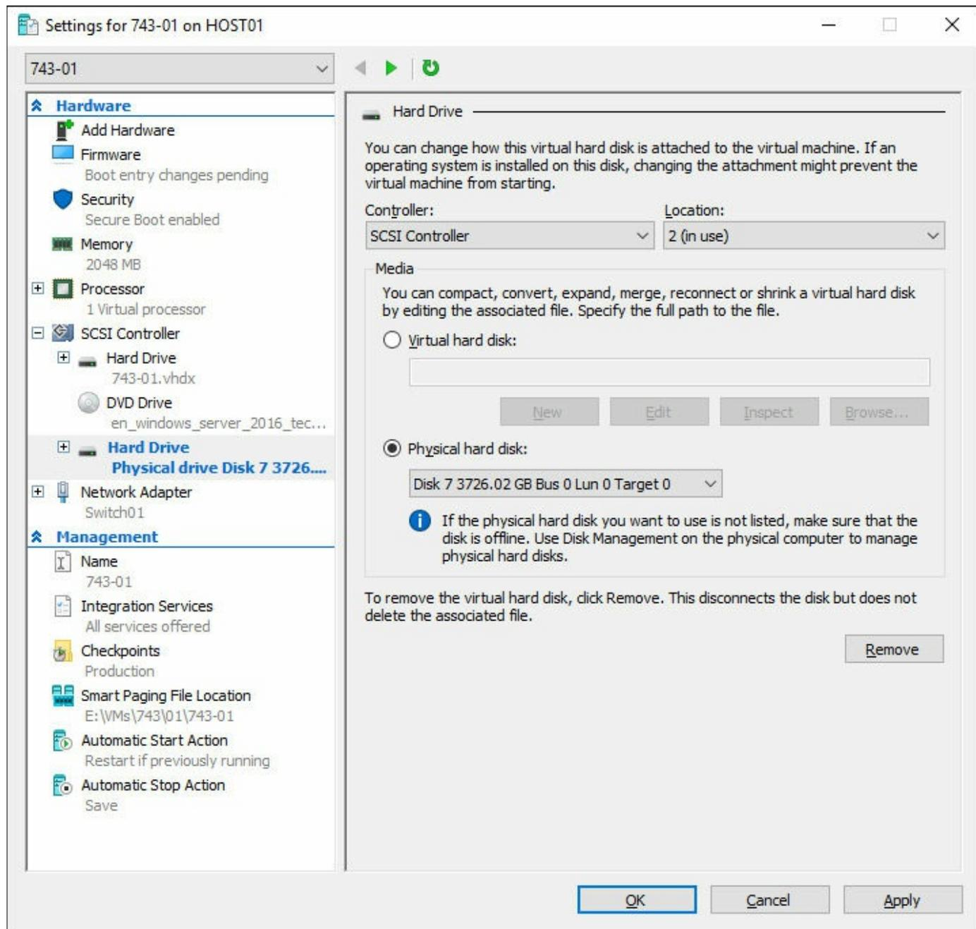
FIGURE 3-18 Adding physical hard disk to a VM
