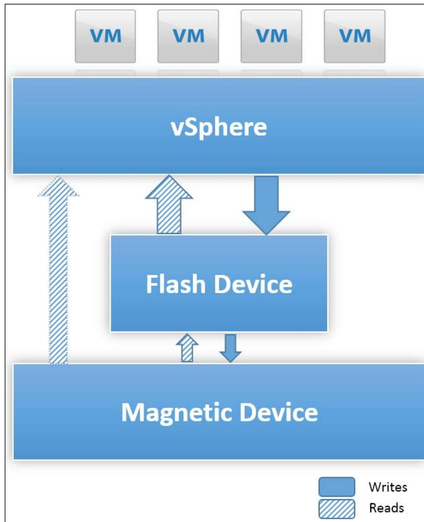
A flash device or solid state disk is an electronic disk; ironically, there is no real "disk" that spins. The data is persistently stored through integrated circuit assemblies. The interfaces to SSD are still compatible traditional block I/O disk drives, which make it easier to replace/swap/interchange HDDs with SSDs.
