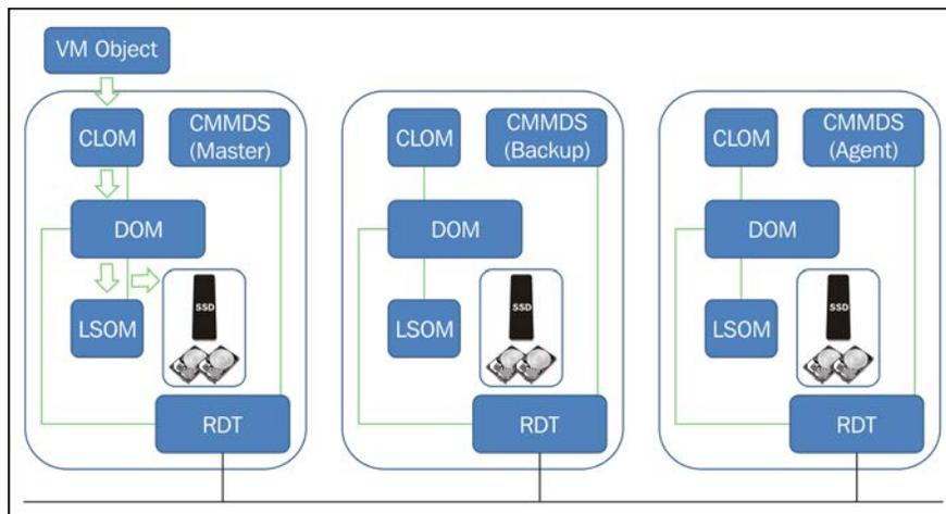
The preceding block diagram outlines the structure of the internal components of VSAN. This is the workflow through which CLOM validates resource availability and DOM creates components and applies configuration locally through LSOM and coordinates with counterparts for component creation on other nodes.
