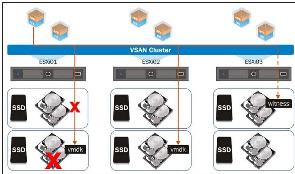
In the preceding example, assume the virtual machine is configured with failure to tolerate as 1. One of the magnetic disks in the disk group that happened to hold a component of the object has failed. The I/O that is directed towards this failed component is then redirected to its counterpart.
