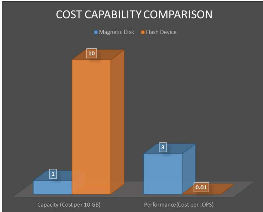
It's not rocket science to realize that the capacity of a magnetic disk is fairly cheap and the cost of IOPS is exponentially cheaper for an SSD.
