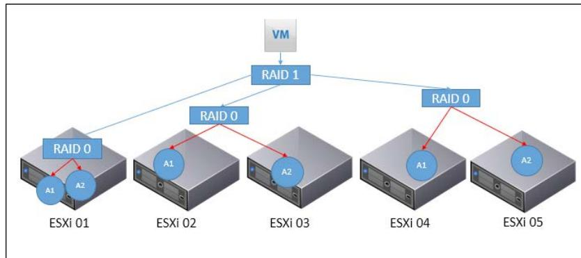
An administrator can validate the actual physical disk placement of the components, that is, the parts that make up the object from the virtual machines' **Manage** tab from the vSphere web client. Navigate to **VM | Manage | VM Storage Policies**:
