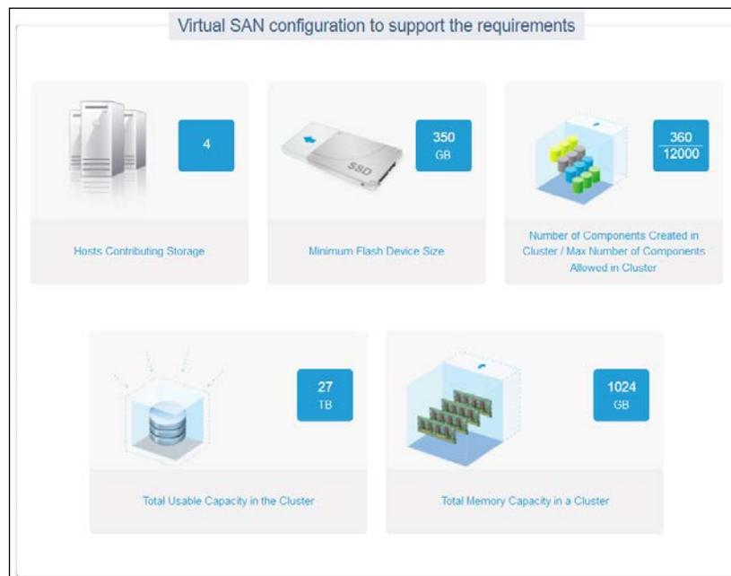
In this example, based on the user inputs as requirements, the proposed design for the VSAN cluster will require four hosts contributing storage. The total usage capacity in the cluster is 27 TB and the minimum flash device capacity per disk group is estimated to be 350 GB. The preceding scenario is an example with random inputs.
