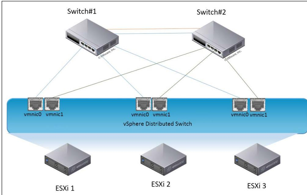
The following is the vSphere Distributed Switch configuration:
