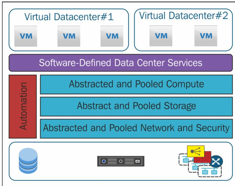
To understand SDDC, we must start by clarifying that it is not a data center controlled merely by automation or scripting. As depicted in the previous figure, it is rather the creation of abstraction layers for compute, storage, network, and security that are managed at the software layer on top of which virtual data centers are built and scaled.
