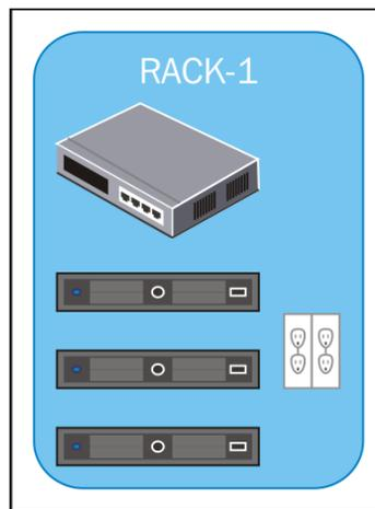
Let's discuss this with the help of an example. A virtual machine with FTT ( $n$ ) set to 1 requires  $2n+1$  number of hosts; three hosts to sustain failures if the fault domain is enabled in the cluster. The VSAN logic will ensure that the objects are distributed on hosts across multiple fault domains, even if there are multiple hosts available on a single fault domain. The following image demonstrates server distribution across racks and the fault domain definition.
