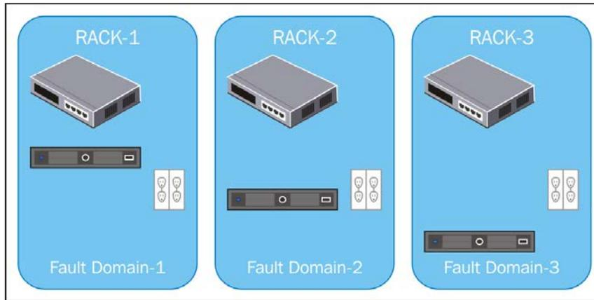
In a similar fashion, with the increasing values of FTT, the number of fault domains should increase as per the  $2n+1$  rule. In short, the failures of all hosts under a single fault domain is considered to be a single failure, similar to one host failure in the context of FTT.
