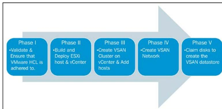
The phases in an installation workflow are as follows:
