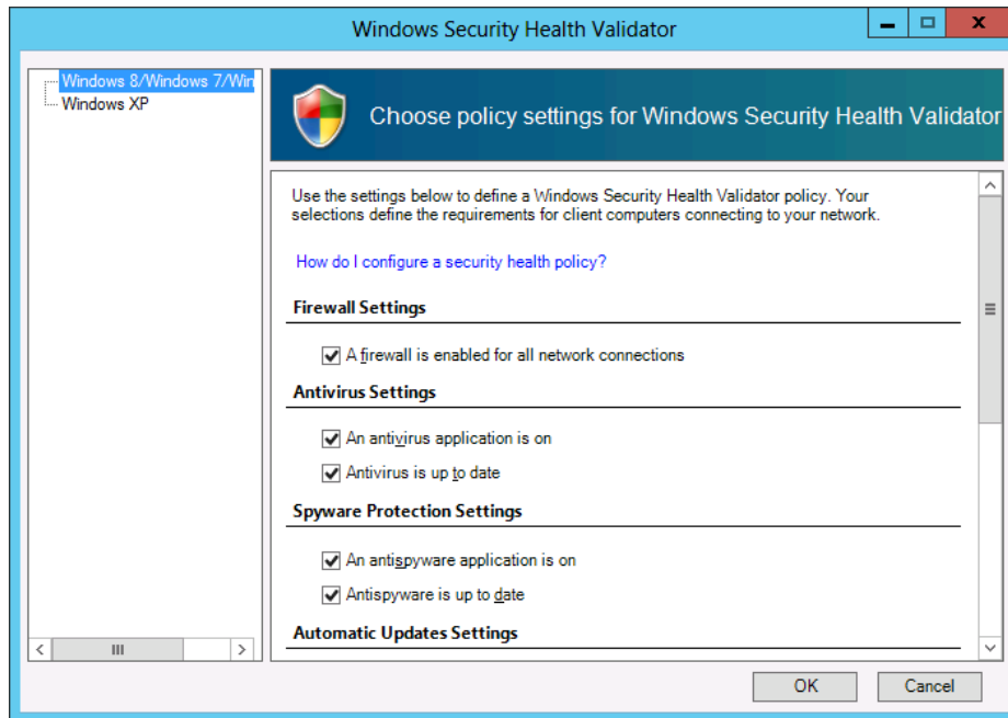
FIGURE 7-7 Specifying settings for a new SHV configuration
