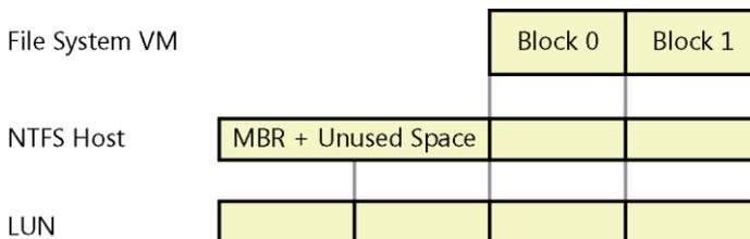
The following block diagram shows a file system misalignment problem what will result in bad performance. Every block that is accessed by the operating system of the virtual machines requires the LUN to access two blocks. This doubles the I/O load on your SAN:
