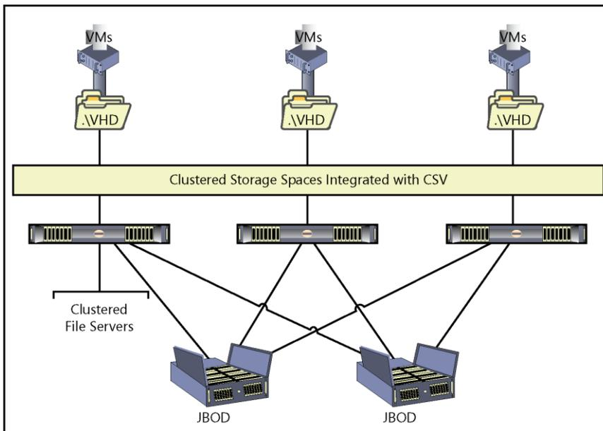
With SSDs in enclosures we would be looking at millions of IOPS from the solution with only the server CPU and storage controllers being the bottleneck. Once we saturate the solution, we can scale out by adding more servers or JBODs.
