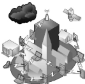
Figure 7.3 Instant formation of ad hoc network in a city during disaster recovery operation.
