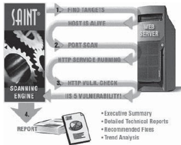
**Figure 1-17** SAINT is a scanning engine that attempts to protect live systems, such as Web servers.
