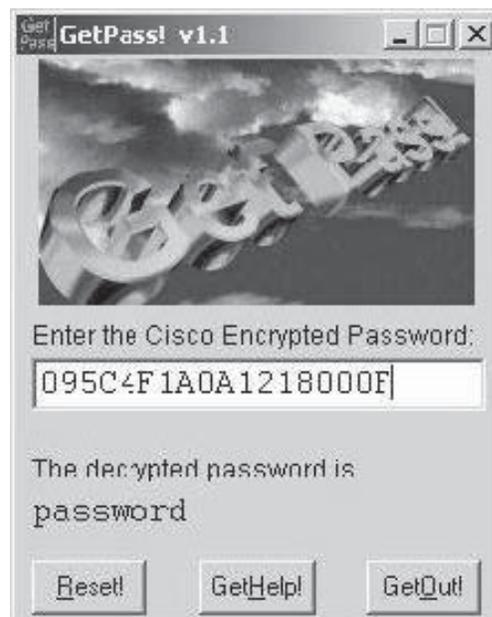
**Figure 3-8** GetPass! can decrypt a Cisco password.
