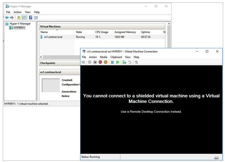
FIGURE 2-4 Here we see that Hyper-V Manager doesn't display a thumbnail preview of a shielded VM, and you also receive an error message when you attempt to start a local connection to the VM
